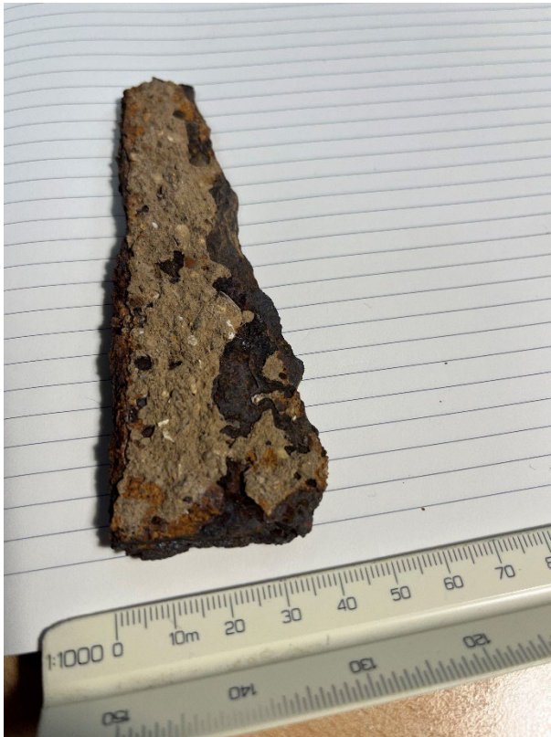
Photograph of a section of the strap remove from the bed joint.
